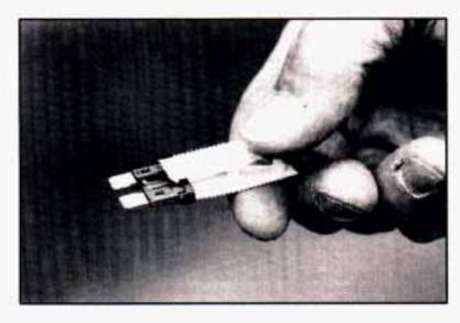
You can remove fuses with a fuse extractor.
